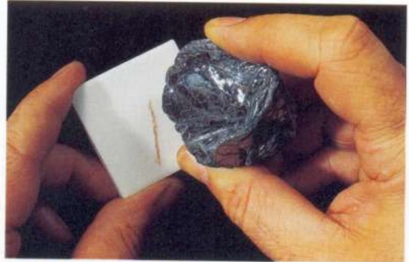
**Figure 3.18 Streak of a Mineral** Color contrast between hematite mineral specimen and a hematite streak. Massive hematite is opaque, has a metallic luster, and appears black. On a porcelain plate, hematite gives a red streak.
